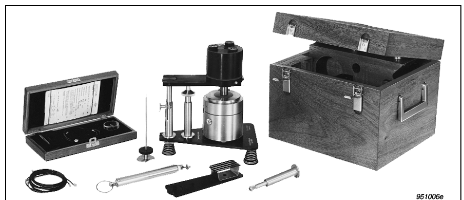
Fig. 7 Artificial Mastoid with calibration set-up
